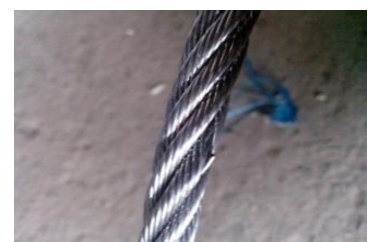
Broken wire rope
