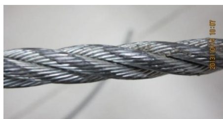
Worn out wire rope
